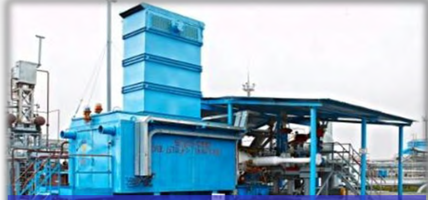
Expander-generator units for NG and AG treatment and Power Generating Units
