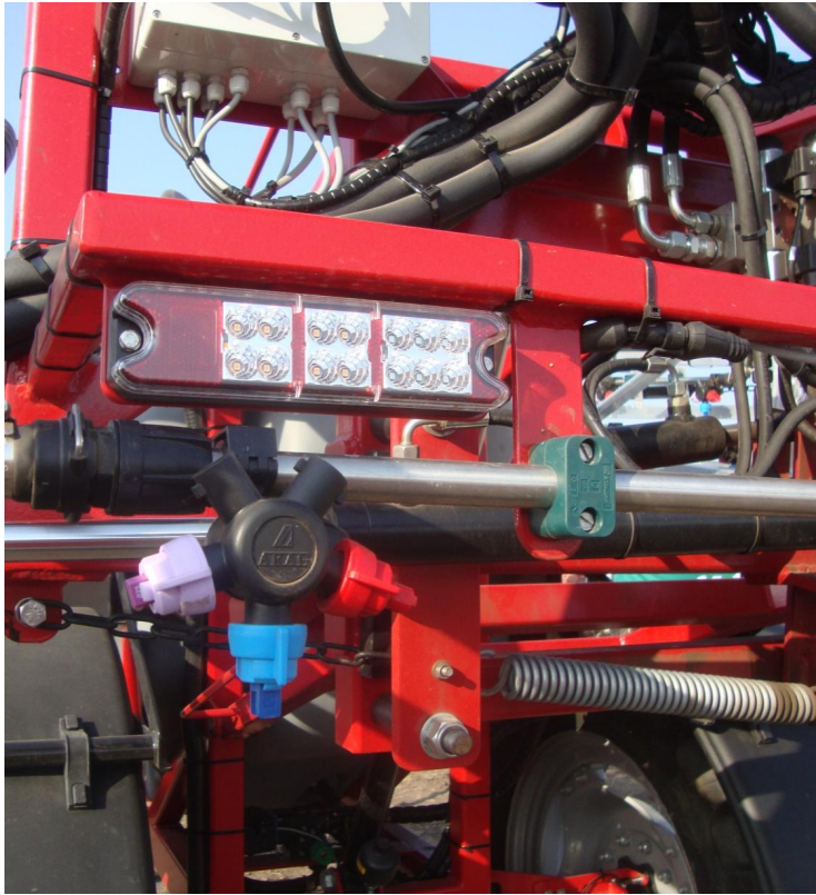
Five nozzle head protected by a boom frame
